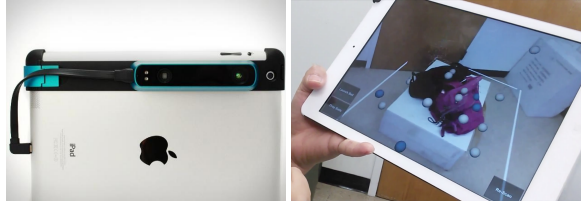
Figure 2: A 3D Structure Sensor attached to a tablet (left) and a physical simulation interface (right) are used in this paper. The interface simulates a few balls falling onto a bag.
