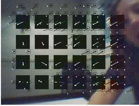
Figure 2: Debug visualization of the vid.stab library (Martius, 2014) showing blocks with sufficient contrast and estimated vectors.
