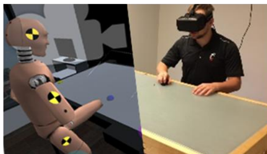
Figure 1: Illustration of experimental setup. At the beginning of each trial a virtual disc would appear on the left side of the table within the appearance range. Disc color indicated target location for that trial. The targets squares (M = magenta, Y= yellow, G = green, B = Blue, R = red) were always visible on the right side of the table. test dummy with a height of 1.8m. Both the participants' right hands were represented by a semi-transparent blue sphere at the end of the dummy's right wrist in order to simplify interaction with the task environment. An inverse kinematics
