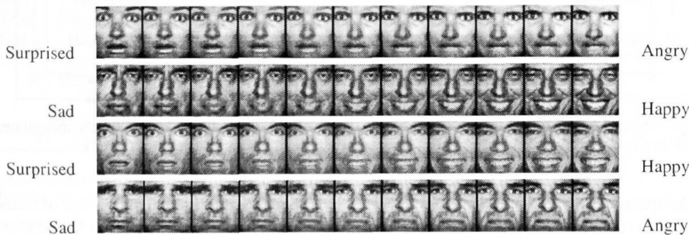
Figure 5: Typical examples of the morphing process. The original expressions are at the extremes of the sequences while the interior images are linear interpolations of the two images.
