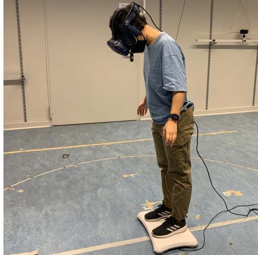
Figure 2: Experimental setup showing the VR and data acquisition devices. Participants stood on the Wii Balance Board while wearing the HTC Vive Pro head-mounted display equipped with the Pupil Labs eye-tracker. Postural sway data were collected using the Wii Balance Board and Microsoft Kinect v2 sensor, placed 2.5 m away at a 37° angle with the anterior direction. Electrocardiography (ECG) was measured using the Polar H10 sensor. The setup was synchronized using the Lab Streaming Layer for accurate multimodal data integration.
