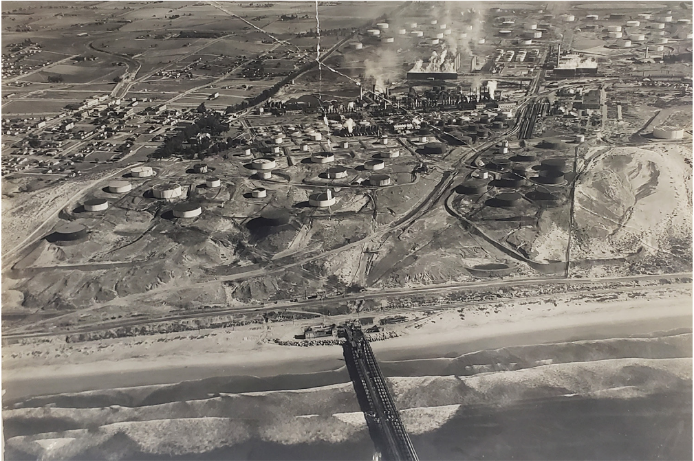
Figure 5. El Segundo Standard Oil Refinery, 1930. "Photo is taken from over the Pacific Ocean looking east at the El Segundo refinery of Standard Oil Company of California (now Chevron). At the bottom of the photo is the refinery's wharf to discharge crude oil and then take on the finished petroleum products for shipment to distant places. To the left of the photo is the emerging City of El Segundo." (El Segundo Historical Society 1930)
