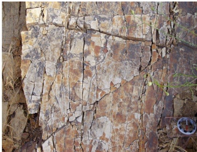
Figure 8. Jointing along the Lower Beacon Trail in Griffith Park. The two prominent joints form a 60^\circ angle. The Silva Ranger Transit in the corner is here for scale (Helman, 2009b).
