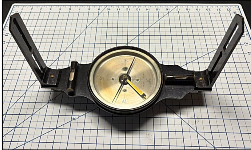
Figure 10. Surveyor's compass made ca. 1880 by John Roach, San Francisco. 11.4 cm (4 ½ in) needle, 1/2° graduations, in quadrants.
