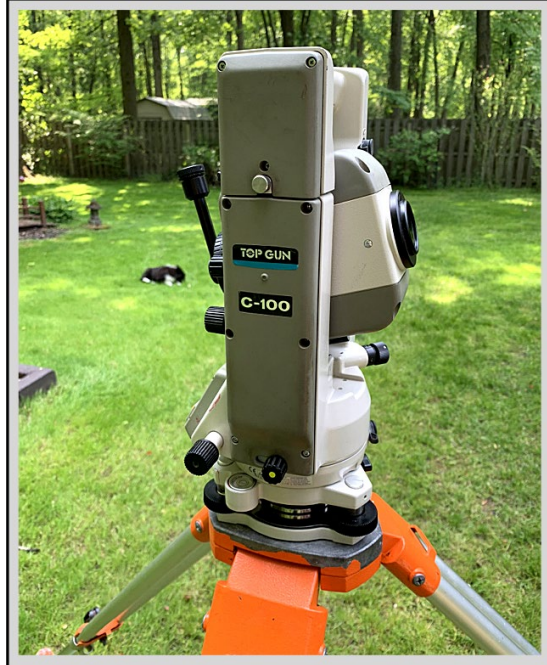
Figure 16. Nikon C-100 total station with attached solar filter and right-angle viewfinder. Photo by author.
