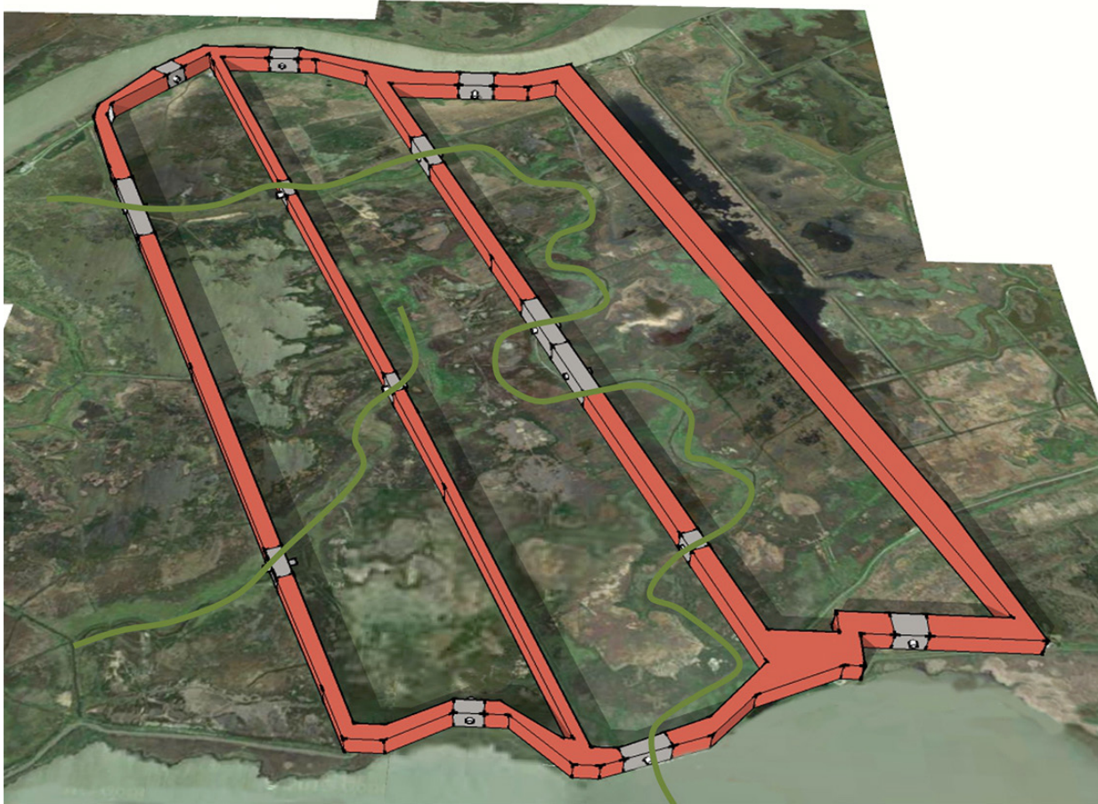
Figure 10 Dike and gate configuration so support one-way flows across replicate ponds, or tidal, two-way flows along historic slough pathways
