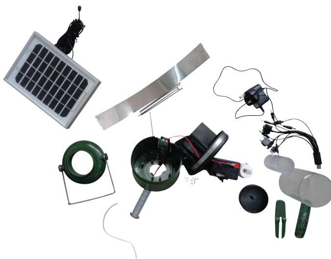
Disassembled powerpoint solar powered lantern.
