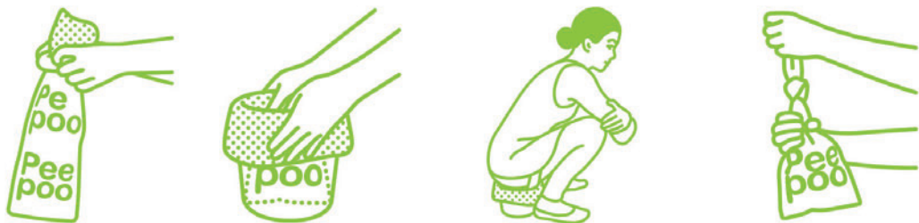
THE PEEPOO TOILET: "Peepoo is designed to be used once, while sitting, squatting or standing. For more convenience, Peepoo can also be placed on the Peepoo Kiti or on a small bucket and used as a chamber pot. Because Peepoo is small, lightweight and not fixed in place, it can easily be used indoors or carried to a secluded spot for use as a private toilet."
