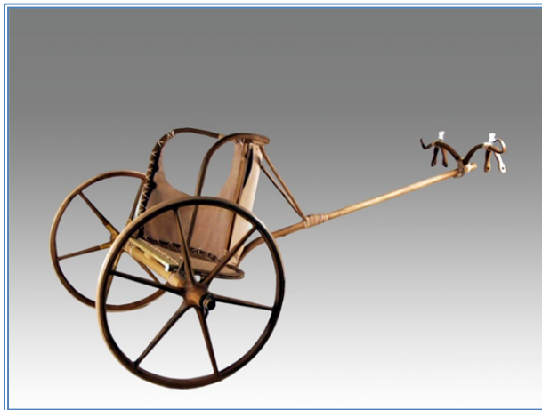
Figure 4. Replica of an Egyptian chariot, based on the chariot in the Museo Egizio de Firenze (no. 2678) and those from the tomb of Tutankhamen.
