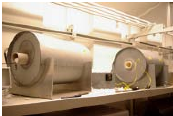
Figure 4. Two of several high-temperature furnaces for solid-state reactions.
