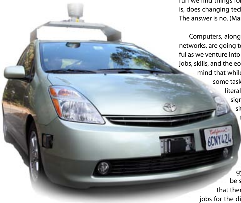
Figure 3. One of eight self-driving cars, this Toyota Prius is one being tested by Google's autonomous car team.
