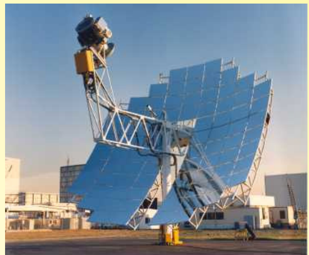
The combination of parabolic reflectors and a Stirling heat engine can produce efficiencies upward of 30%, almost double that of competing photovoltaic technologies. These so-called "Dish-Sterling" or "Solar-Sterling" systems provide the highest known efficiencies of any method.
