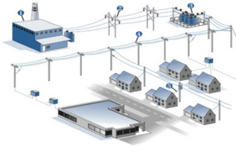
Figure 6. Micro-synchrophasors ( \mu PMU's) at every node in a distribution grid
