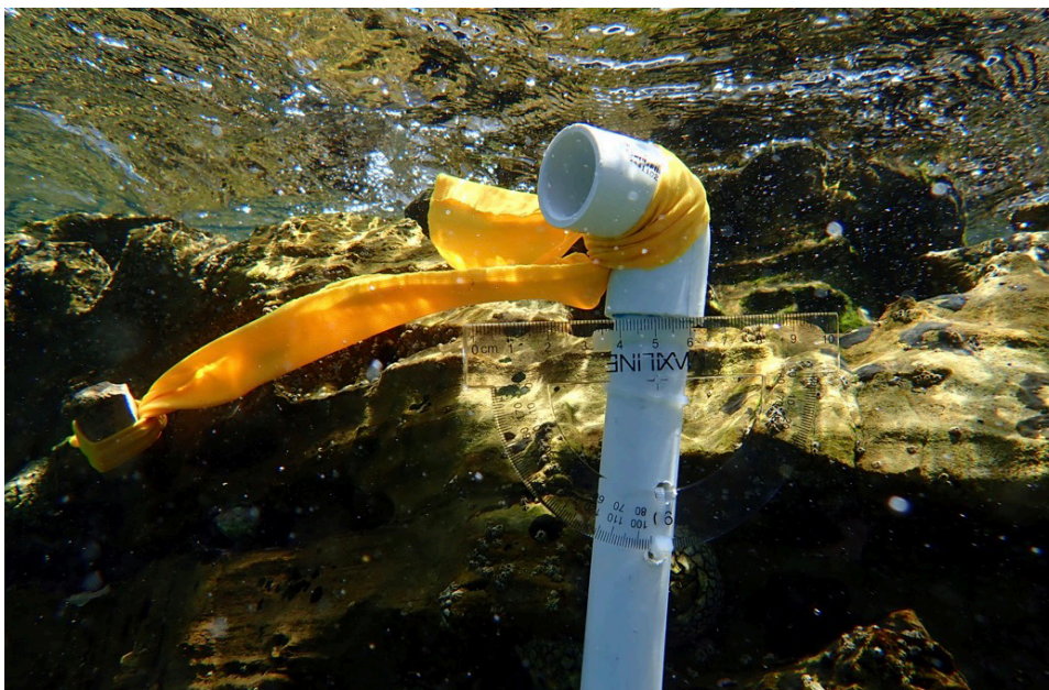
Figure 1. Surge angle tool. A weighted string on a PVC pipe with a protractor was used to measure the surge angle. The highest angle a surge reached was 90 degrees.
