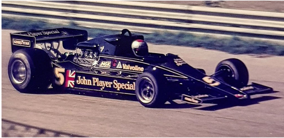
Figure 2: The Lotus 78 was the first car which utilized “ground effect” downforce. The channels on either side of the car led air into large curved surfaces which acted as wings across the entire underside of the car.
