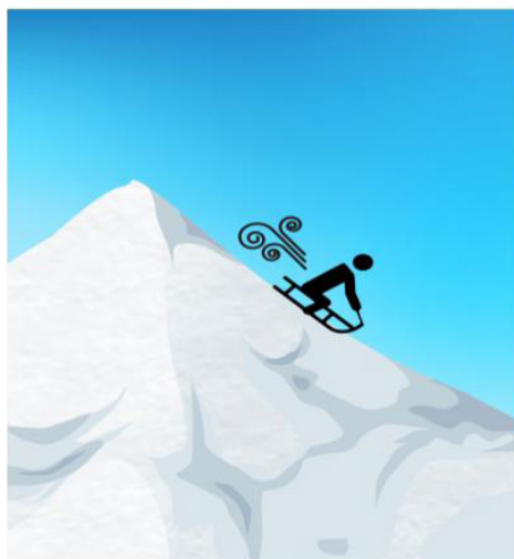
Figure 1b: Imagine a sled on a hill. The potential energy of this system is determined by the hill's height, which, in turn, determines the total kinetic energy the sled will eventually possess. As the sled goes down the hill, its potential energy converts into kinetic energy, which increases as the sled gains velocity. In addition, the friction between the sled and ground converts some of the kinetic energy into heat, and it also converts into the sound one hears as the sled moves. The total energy is conserved in this situation; it just changed into different forms.
