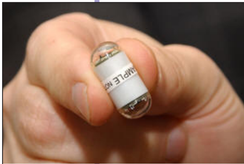
The PillCam pictured is swallowed and used to take pictures of patients' GI tracts to detect diseases.
