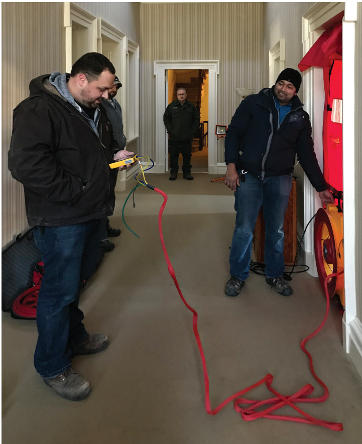
(top row, l-r) FIGURE 7. Indoor particulate monitor. FIGURE 8. Outdoor particulate monitor. DAVID BITTERMANN (bottom row) FIGURE 9. Blower door testing at Lindenwald, Martin Van Buren National Historic Site (left) and at Sagamore Hill National Historic Site (right). MAVA: DAVID BITTERMANN; SAHI: STEVEN WEINTRAUB, ART PRESERVATION SERVICES
