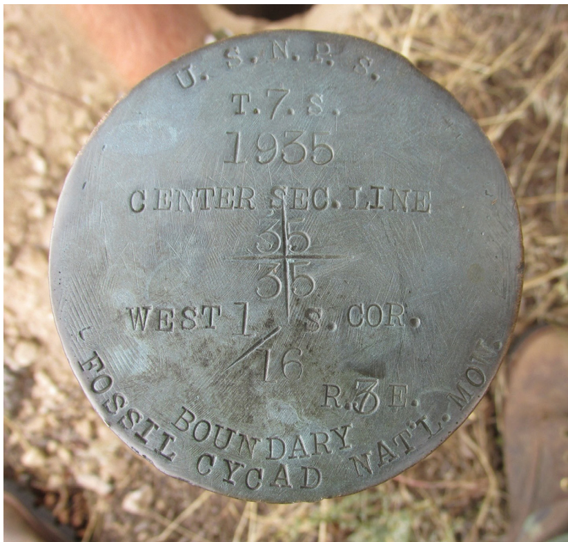
FIGURE 7. One of the boundary survey markers that was installed during the 1930s to delineate the boundary of Fossil Cycad National Monument. It was recently collected to preserve in NPS collections. NATIONAL PARK SERVICE
