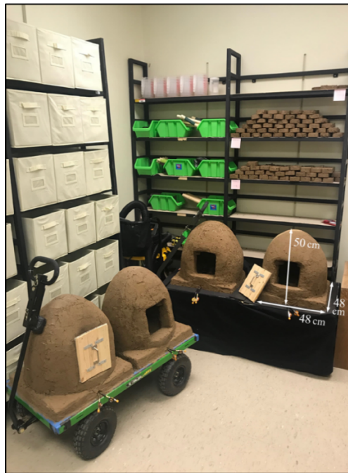
Figure 1. PEARL experimental hornos (bottom) and mini-bricks (middle right) in storage. Photograph by Albert Gonzalez.
