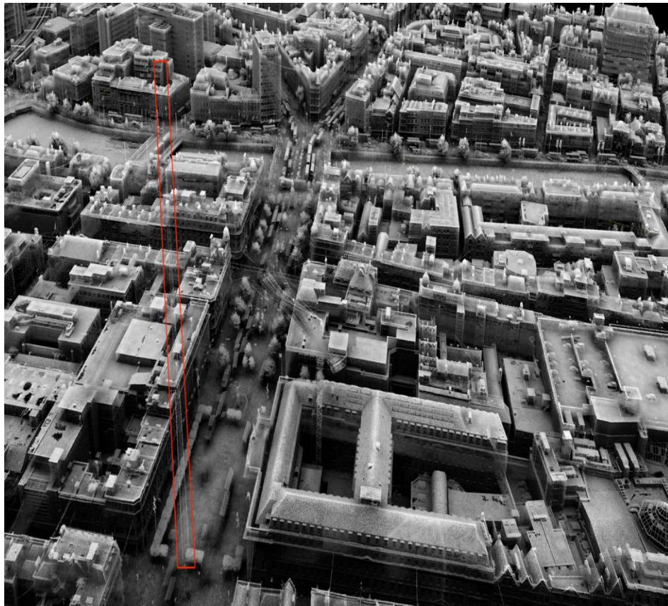
Fig. 7. LiDAR data depicting the height and positioning of The Spire of Dublin (outlined in red) within the enclosed area of O'Connell Street looking south. Digital rendering by Brittney O'Neill and Debra Laefer, 2017.
