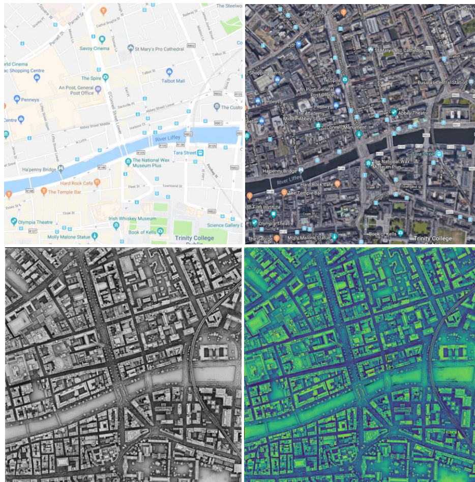
A comparison of representations of central Dublin. Fig. 1 a. (top left) Google maps "Map"; Fig. 1 b. (top right) Google Maps satellite imagery; Fig. 1 c. (bottom left) 3D LiDAR data in grayscale. Fig. 1 d. (bottom right) 3D LiDAR data seen from a God's eye view with intensity values mapped to a viridis color scale. Digital renderings by Brittney O'Neill and Debra Laefer, 2017; Map imagery extracted from Google Maps, 2017.
