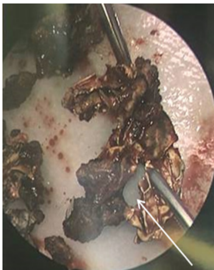
Image 3. Specimen with calcified exterior and synthetic rubbery core indicated by white arrow.
