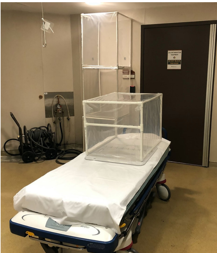
Image 1. Portable respiratory protection unit, constructed of PVC pipe and auto collision wrap, situated on a stretcher in correct position.
