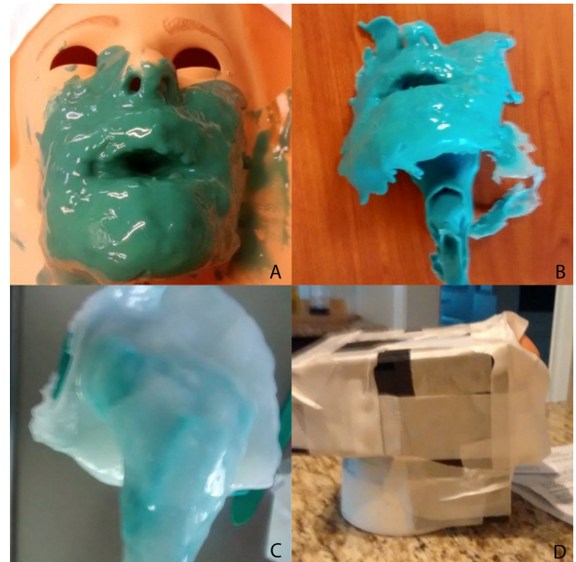
Figure 1. Fabrication of the peritonsillar abscess simulator. A, Casting of the negative mold. B, Negative mold before trimming. C, Casting of the positive mold. D, Scaffold used to make mounting unit.
