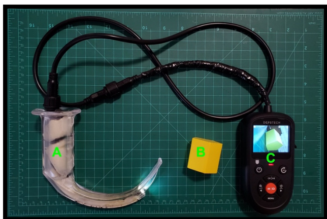
Figure 2: A borescope laryngoscope (A) viewing a yellow block (B) which is displayed on the handheld screen (C).
