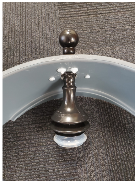
Figure 4: A silicone vacuum suction cup is placed inside the bottom portion of a plunger.
