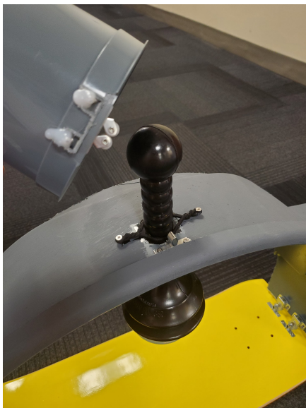
Figure 6: A latch clip is glued on inside portion of a pitcher. It can then be attached to the top portion of the arch and cover the handle of the plunger.
