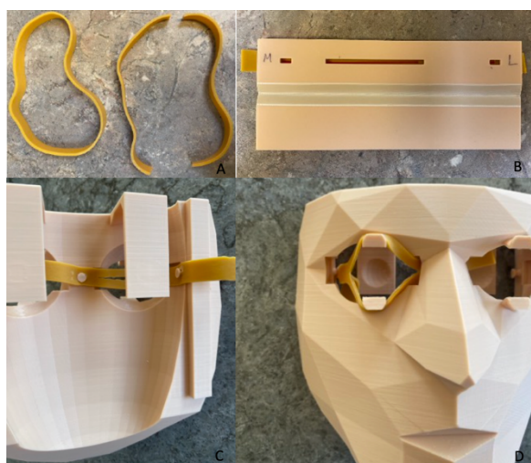
Figure 1. Creation of the lateral canthotomy mask trainer. A. Cut the rubber bands in half. B. Mark rubber bands with 3D printed marker. C. Attach rubber bands to the inner side of mask. D. Attach rubber bands to the outer side of the mask.
