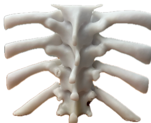
Figure 2. Author's own image. Finalized 3D-printed spine and ribcage model prior to suspension in ballistics gel.
