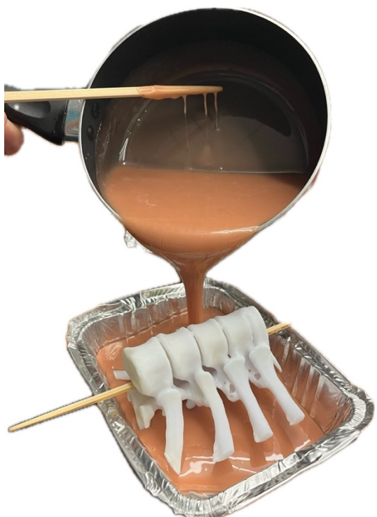
Figure 4. Author's own image. Enough ballistics gel was added, engulfing the ribs completely and leaving the vertebral bodies exposed.
