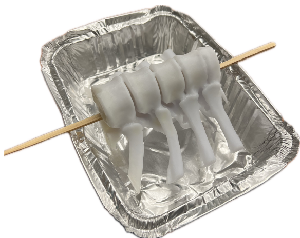
Figure 3. Author's own image. When setting up the 3D printed model, a skewer was inserted through the vertebral foramen. This allows for the ribs to be suspended at a realistic depth when covered by the ballistics gel.
