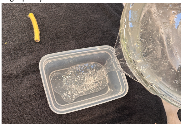
Figure 5: Pouring base layer of ballistics gel into phantom container: Author's own image
