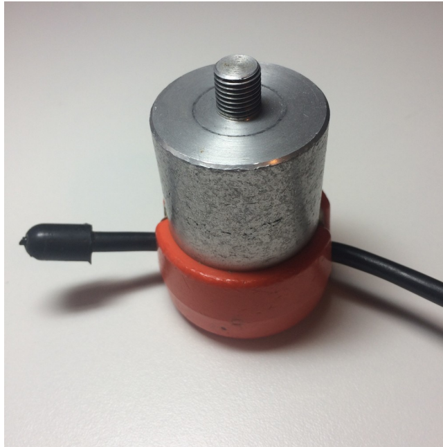
Figure 7. Geophone. The geophone was used as a sensor to determine the capability of the IDS to detect infrasound.
