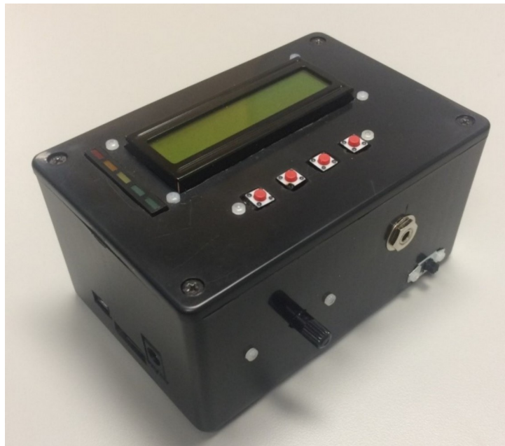
Figure 1. Infrasound Detection System
