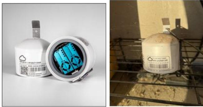
Figure 4. PurpleAir Sensor Serving as the Fixed Monitoring Site at UC Merced: The PurpleAir PA-II-SD sensor (ID 163173) functions as the campus's fixed monitoring site. Left: device with internal optical particle counters exposed. Right: field installation on the exterior of SE2 providing real-time PM 2.5 data for comparison with handheld EXTECH VPC300 measurements.
