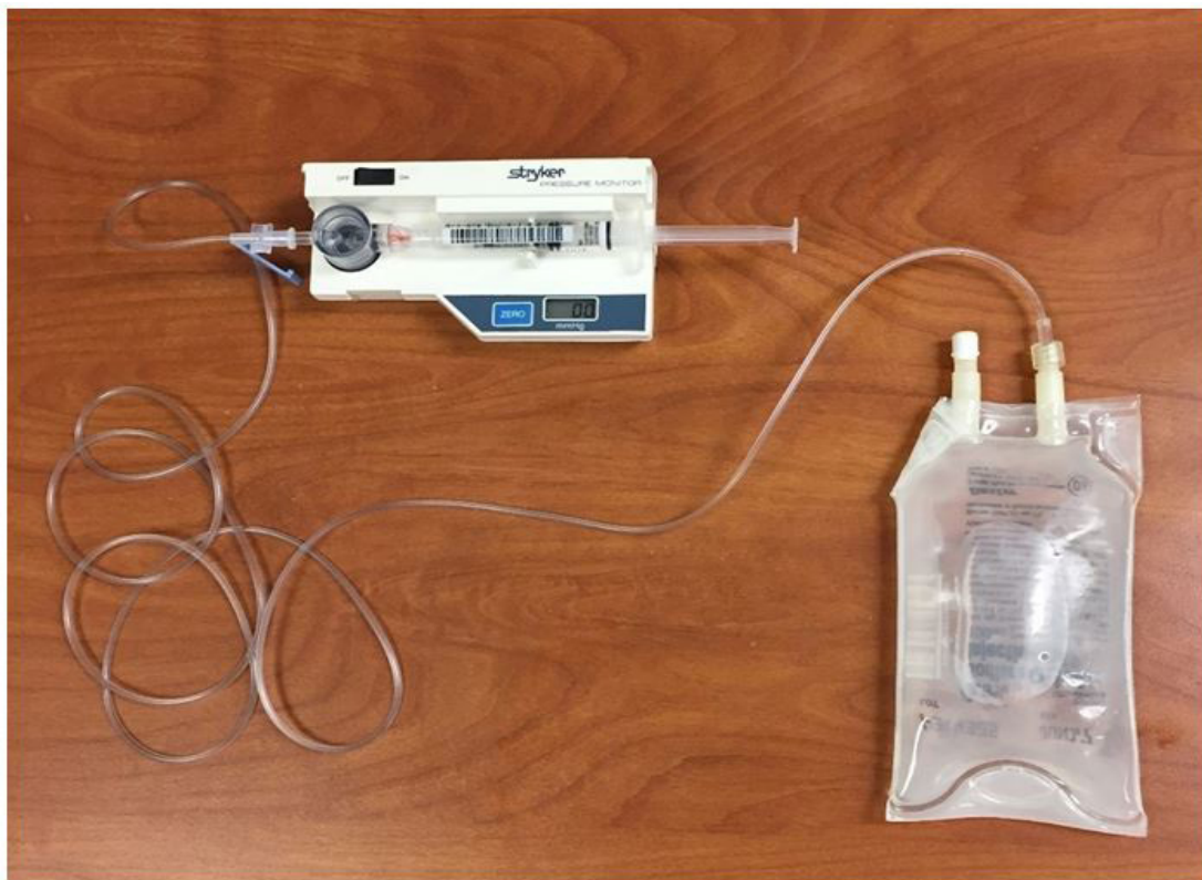
Figure 2. Noninvasive pressure measurement setup, showing 100mL bag of normal saline connected to Stryker pressure meter via standard intravenous (IV) tubing.
