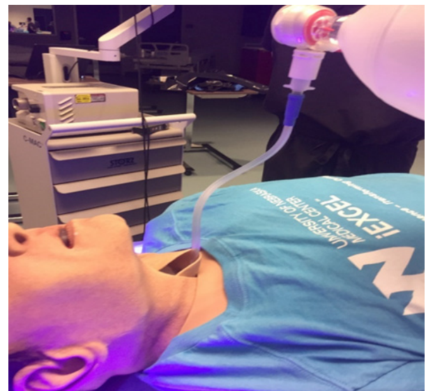
Figure 2. Large Droplet Cough Model using retrograde intubation technique allows for expelled secretions to come directly from mannequin's mouth. BVM used to forcefully expel 5 mL of fluorescent solution. BVM, bag valve mask; mL, milliliter.
