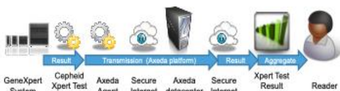
Figure 2. Data flow for cloud-based data aggregation system.
