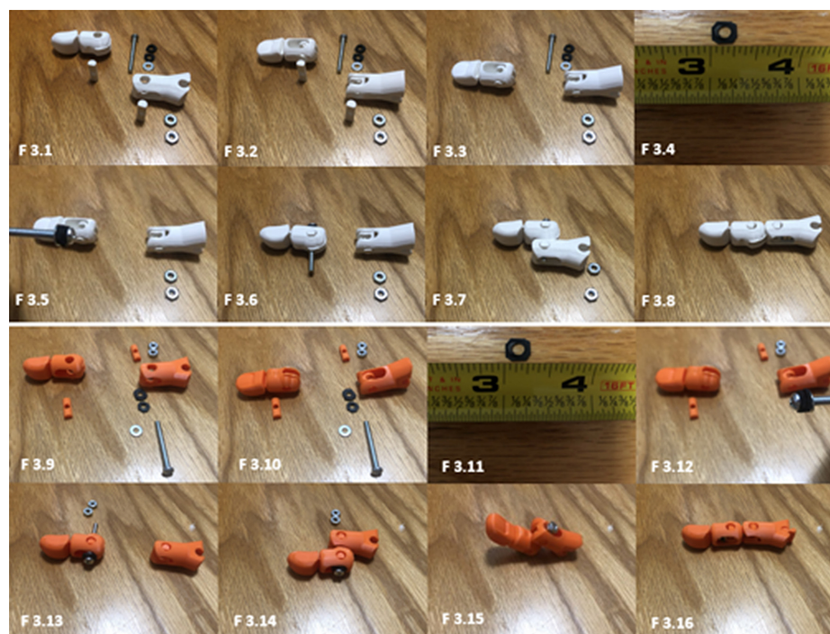
Figure 3. 3.1. Shows all component parts of the dorsally dislocated finger (lateral view). 3.2. Dorsal view. 3.3. Place pin and align the central opening with openings in the middle and proximal finger portions. 3.4. Modified neoprene washer cut \frac{1}{4} in x \frac{1}{4} in. 3.5. Load two neoprene washers and a machine screw nut. 3.6. Load the screw dorsally through the pin. 3.7. Pass screw through pin in proximal phalanges as shown and attach screw nuts in this position. 3.8. Place in the reduced position to check resistance. 3.9. Shows all component parts of the volar dislocated finger (lateral view). 3.10. Dorsal view. 3.11. Modified neoprene washer cut \frac{1}{4} in x \frac{1}{4} in. 3.12. Load two neoprene washers and machine screw nut. 3.13. Load the screw ventrally through the pin. 3.14. Pass screw through pin in proximal phalanges as shown and 3.15. attach screw nuts in this position. 3.16. Place in the reduced position to check resistance.
