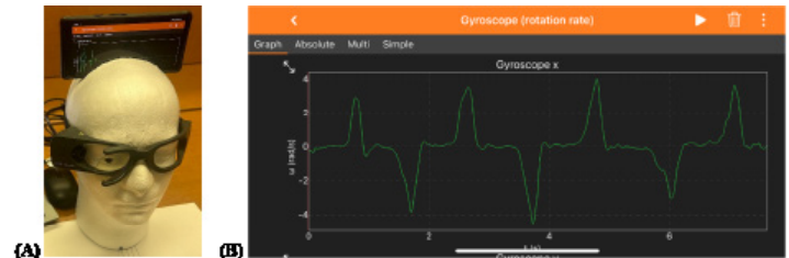
Figure 1. (A) Training model with video-oculography (VOG) device and smartphone placement. (B) Interface of the smartphone application displaying rotational velocity.
