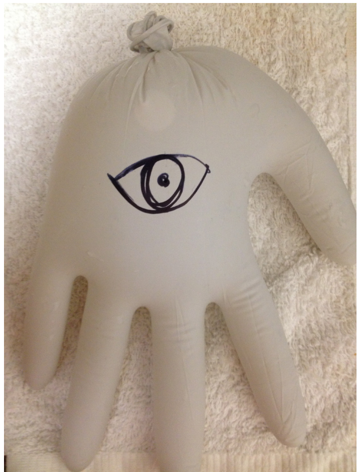
Figure 4. Eye model made of glove filled with water.
